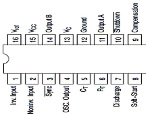
Figure 6. SG3525 pin connections [9].
