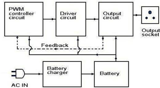
Block diagram of a basic PWM inverter www.circuitstoday.com
