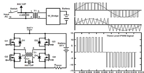
Figure 4. Inverter Mode Gate Drives [10].
