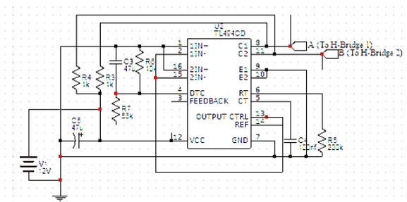
Figure 8. Designed Circuit of the DC-AC Oscillator
