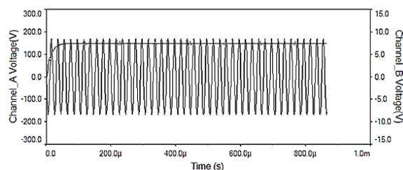
Figure 11. Simulation result on the bridge rectifier circuit
