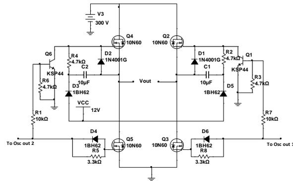
Figure 9. The Designed High Bridge Driver Circuit.
