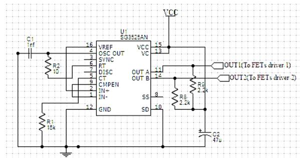
Figure 7. Designed circuit of the DC-DC Oscillator
