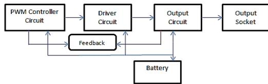
Figure 5. Block diagram of the setup.
