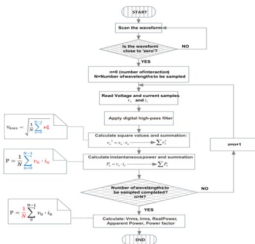
Figure 8: Power calculation subroutine flow diagram
