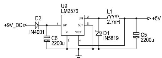
Figure 6. Power Supply Circuit [10].
