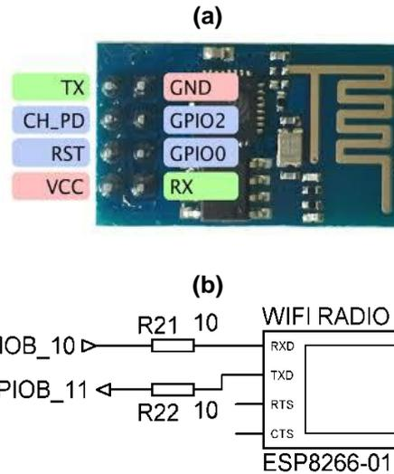
Figure 4 (a). ESP8266-01 Wi-Fi Module and (b). ESP8266-01 Wi-Fi Module Connection
