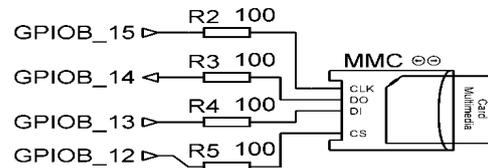
Figure 5: SD Card Connection
