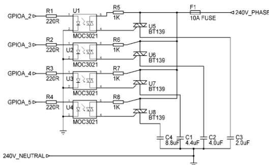
Figure 3. Capacitor Bank Switching Circuit
