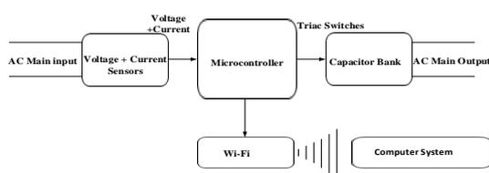
Figure 1. Functional Block Diagram of the Power Factor Monitoring and Correction System
