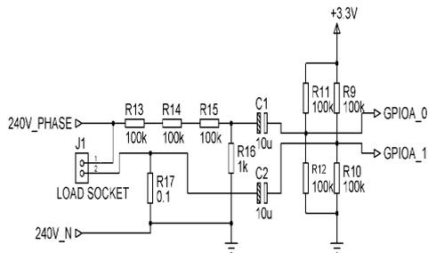
Figure 2. Voltage and Current Sensing Unit
