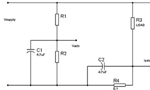
Figure 2. Voltage Divider Attenuator Circuit
