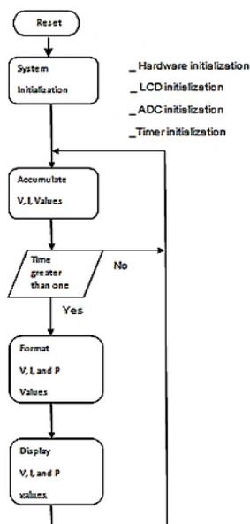
Figure 1. Voltmeter, Ammeter and power Flow Chart.
