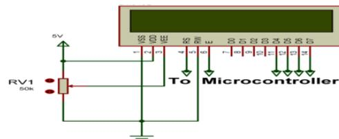
**Figure 3.** Liquid Crystal Display Circuit Diagram source: [7]
