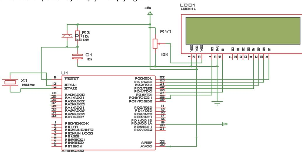
**Figure 4.** The Designed Circuit Showing PIC and LCD Connections
