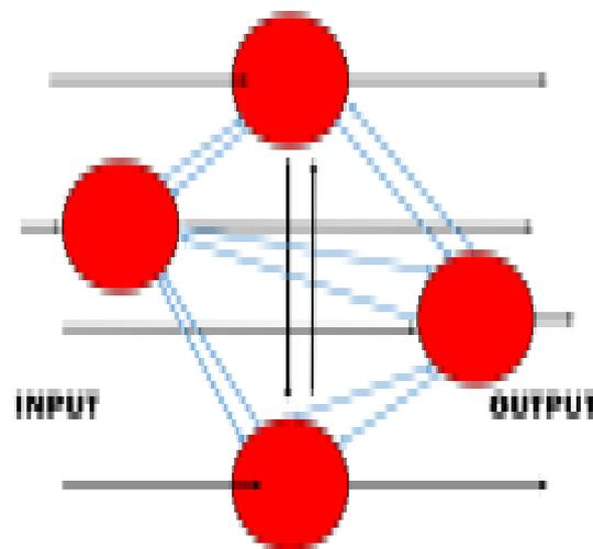
Figure 1. Simple Topology of Hopfield Neural Network
