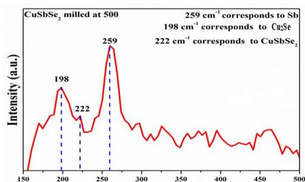
**Fig. 2:** Typical Raman spectrum for as-milled  $\text{CuSbSe}_2$
