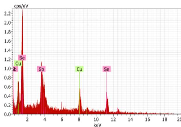
**Fig. 4:** EDS spectrum of as-milled  $\text{CuSbSe}_2$
