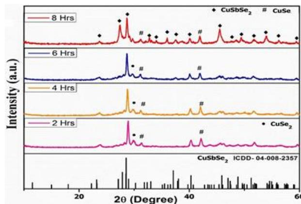
Fig. 1: Typical XRD pattern for as-milled CuSbSe<sub>2</sub>
