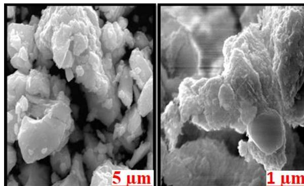
**Fig. 3:** FE-SEM micrographs of the wet as-milled (8 hours) sample
