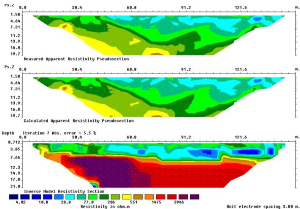
Figure 4: Inverse Model of Resistivity Section
