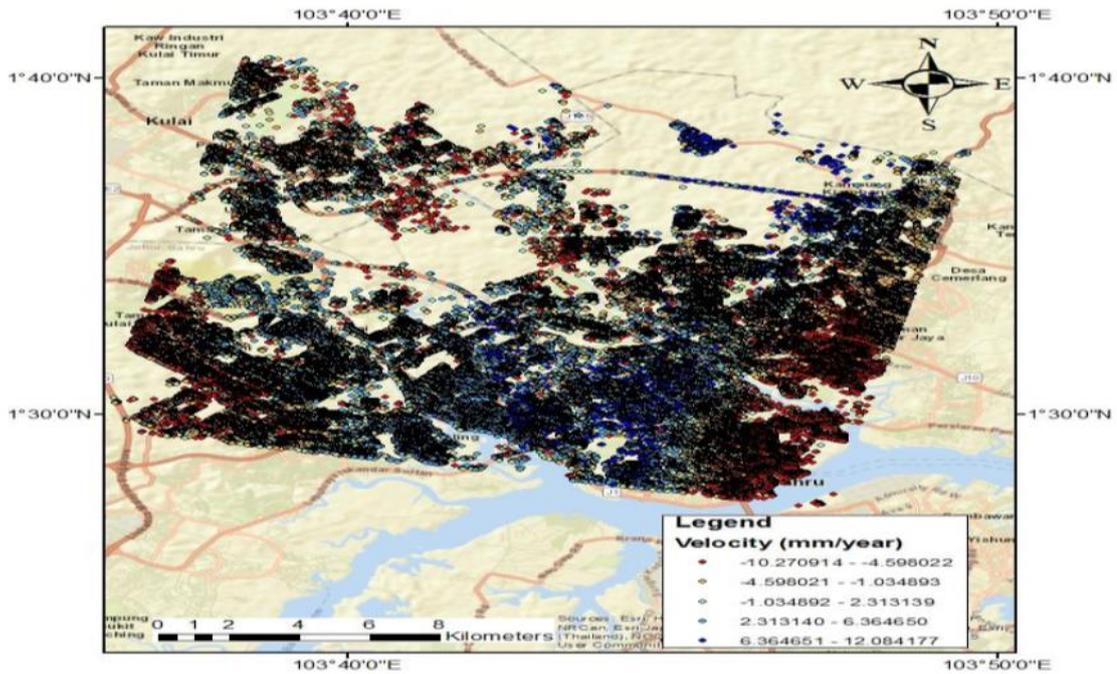
Figure 3: Persistent Scatterer Interferometry Map showing Ground Displacement.
